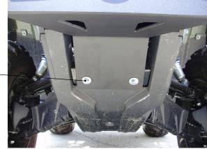
SLIDE THE MAIN BUMPER OVER THE MOUNTING BRACKET USE SIX OF THE CARRIAGE HEAD BOLTS WASHERS AND LOCK NUTS.-
