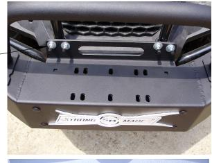
SECURE THE BOTTOM OF THE MOUNT WITH THE TWO 5/16 X 1 BOLTS FOUR 5/16 USS WASHERS AND TWO LOCK NUTS.
