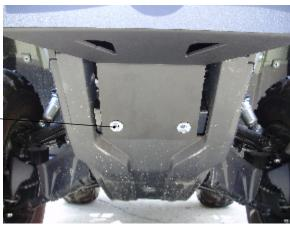
SLIDE THE MAIN BUMPER OVER THE MOUNTING BRACKET USE SIX OF THE CARRIAGE HEAD BOLTS WASHERS AND LOCK NUTS.-
