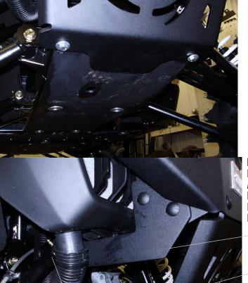
INSTALL THE OUTER SIDE BRACKETS ON LEAVE ALL HARDWARE LOOSE. THERE IS A RIGHT AND LEFT WHEN MOUN TING THE BRACKETS.USE THE 5/16 BOLTS WASHERS LOCK NUTS. ALSO REMOVE THE TOP CONTROL ARM BOLT REPLACE IT WITH THE SUPPLIED 80MM BOLT AND LOCK NUT.
