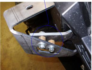
3RD STEP: INSERT THE 5/16X1 1/4 U-BOLT AROUND THE PIPE ON FRAME. USE 2=5/16 USS WASHERS 2=5/16 LOCK NUTS. REPEAT ON THE OPPOSITE SIDE.
