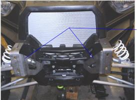
**1ST STEP: REMOVE THE PLASTIC** RADIATOR GUARD AND BOTTOM ACCESS PANEL. TOP CAN BE REPLACED ONCE BUMPER IS MOUNTED. BOTTOM CAN ALSO WITH A LITTLE TRIMMING OF PLASTIC. INSTALL THE LEFT AND RIGHT BRACKETS WITH 3/8X1 BOLT 2=3/8 WASHERS AND 2=3/8 NUTS.
