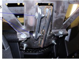
TUBING ROLL BAR WILL MOUNT ONTOP OF THE BUMPER AFTER ALL BRACKETS AND BUMPER COVER ARE INSTALLED. USE FOUR OF THE CARRIAGE HEAD BOLTS WITH WASHERS AND LOCK NUTS TO MOUNT THE BAR TO BUMPER COVER.
