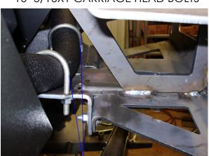
LEAVE ALL HARDWARE LOOSE UNTIL ALL BRACKETS ARE INSTALLED AND CENTERED.
