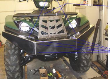
LAST STEP: MOUNT THE TOP OF THE LARGE BRACKET TO THE RACK USE THE 1/4X1/2 U-BOLTS 1/4 USS WASHERS AND 1/4 LOCK NUTS HERE. ONCE BRACKETS ARE CENTERED, TIGHTEN ALL HARDWARE. LAST SLIDE THE BUMPER COVER OVER THE BRACKETS AND SECURE IT TO THE BRACKETS WITH THE CARRIAGE HEAD BOLTS 5/16 USS WASHERS AND 5/16 LOCK NUTS.
