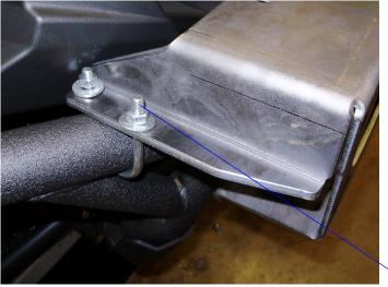
2ND STEP: PLACE THE U-BOLTS AROUND THE BUMPER PIPE AND THROUGH THE OVAL HOLES ON THE TOP OF THE BRACKET. PLACE WASHERS AND LOCK NUTS ONTO THREADS LEAVE LOOSE UNTIL ALL HARDWARE HAS BEEN PLACED IN CORRECT
