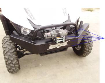
LAST STEP: SLIDE BUMPER COVER OVER MAIN BRACKET AND SECURE IT TO MAIN BRACKET. USE THE CARRIAGE HEAD BOLTS WITH WASHERS AND LOCK NUTS. THE GRAB BAR WILL ALSO USE THE CARRIAGE HEAD BOLTS WITH WASHERS AND LOCK NUTS. TIGHTEN ALL HARDWARE THAT WAS LEFT LOOSE EARLIER.
