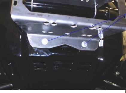
LAST SLIDE THE BUMPER COVER OVER THE BRACKET. USE THE 5/16 CARRIAGE HEAD BOLTS AND 5/16 USS WASHERS WITH 5/16 LOCK NUTS TO MOUNT TO THE BRACKET. - PLACE ONE IN EACH OF THE SIX SQUARE HOLES. THE WINCH WILL COME WILL ITS OWN HARDWARE TO MOUNT TO THE BUMPER.
