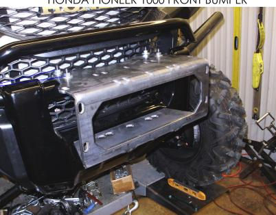
USE THE 5/16X1 BOLTS WITH 5/16 USS WASHERS AND 5/16 LOCK NUTS HERE.
