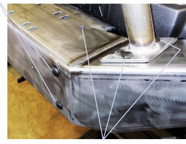
USE THE 5/16X1 CARRIAGE HEAD BOLTS HERE TO FINISH THE MOUNTING. THEN PROCEED TO TIGHTEN ALL HARDWARE.
