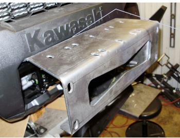
2:ND INSERT THE SIDE BRACKETS INTO THE FRAME THERE IS A RIGHT AND LEFT SIDE TO THESE. SECURE THESE TO THE FACTORY FRAME WITH TWO U-BOLTS WITH WASHERS AND LOCK NUTS. AGAIN LEAVE LOOSE.
