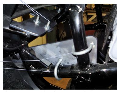
LAST ONCE BUMPER BRACKETS ARE IN PLACE SLIDE THE BUMPER COVER OVER THE BRACKETS AND INSERT THE 5/16X1 1/4 CARRIAGE HEAD BOLTS THROUGH THE FRONT INTO ALL PLATES SECURE WITH 5/16 USS AND 5/16 LOCK NUTS.
