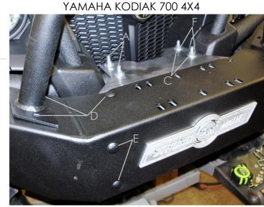
2ND STEP SLIDE THE LEFT AND RIGHT BRACKET INTO PLACE AND LOOSELY SECURE IT WITH THE 1/4 X 3/4 U-BOLTS 1/4 WASHERS AND LOCK NUTS.
