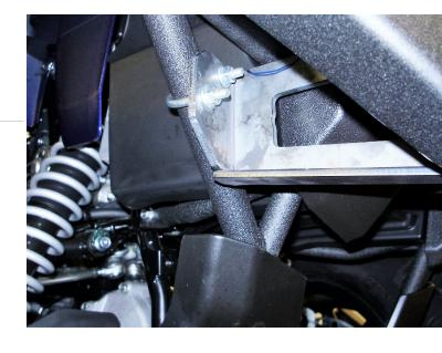
THIS IS A FINAL PIC ON THE BUMPER ONCE INSTALLED WITH A 3000LB WINCH BUT YOU WILL HAVE TO USE A ROLLER PLATE AND A FAIRLEAD FOR THE CABLE.
