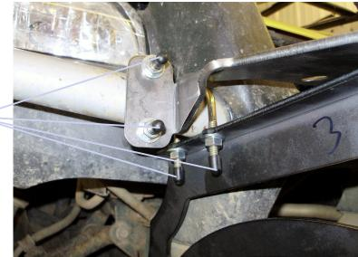
PLACE THE 1/4 ROD CAPS ON ALL 1/4" EXISTING THREADS AFTER ALL HARDWARE IS TIGHTENED.
