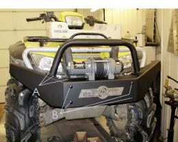
LAST SLIDE THE MAIN BUMPER COVER ON AND INSERT THE 1" AND 1 1/4 LONG CARRIAGE HEADS INTO THE SQUARE HOLES. THEN PROCEED TO TIGHTEN ALL HARDWARE.
