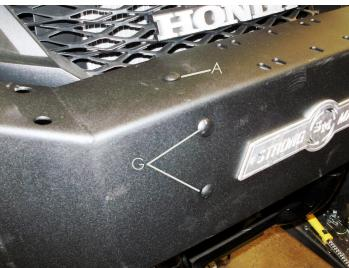
SLIDE THE FRONT BUMPER COVER ON AFTER ALL BRACKETS ARE IN PLACE. INSERT THE CARRIAGE BOLTS WITH WASHERS AND LOCK NUTS ON.
