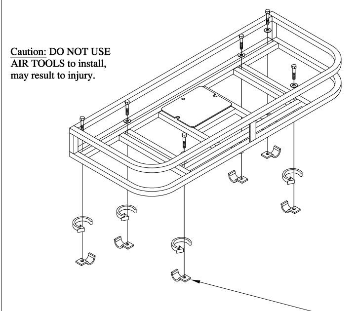
THE CLIPS WILL MOUNT EITHER WAY DEPENDING ON THE ORIGINAL RACK DESIGN.
