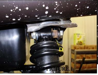
INSTALL THE SWAY BAR BRACKETS USING THE TWO 8MM X 40MM BOLTS AND 5/16 SAE WASHERS. INSTALL ON EACH SIDE.
