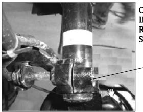
ONCE THE SPRING HAS BEEN INSTALLED ONTO THE SHOCK, REINSTALL THE SHOCK INTO THE STEERING KNUCKLE.
