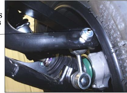
THIS IS PIC OF THE FRONT LEFT SIDE MOUNT. THIS KIT WILL MOUNT TO THE TOP OF THE SHOCK ON THE FRONT, REPEAT THE SAME FOR THE FRONT RIGHT SIDE TO INSTALL.
