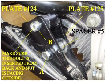
WHEN INSTALLING PLATES AND BRACKETS LEAVE ALL FASTENERS LOOSE UNTIL ALL HARDWARE IS IN PLACE THEN PROCEED TO SECURE THE KIT. AFTER INSTALLATION MAY HAVE TO ADJUST THE TIE RODS TO CORRECT THE ALIGNMENT OF THE WHEELS. IF BOOT GUARDS ARE INSTALLED MUST CHECK FOR PROPER CLEARANCE FOR THE RIMS AND BRAKE CALIPERS. TO CHECK FOR THIS LIFT THE FRONT OF THE ATV OFF THE GROUND AND TURN WHEELS FROM LEFT TO RIGHT AND MAKE SURE NOTHING IS TOUCHING THE GUARDS. MAY HAVE TO TRIM MATERIAL AWAY FROM THE GUARDS
