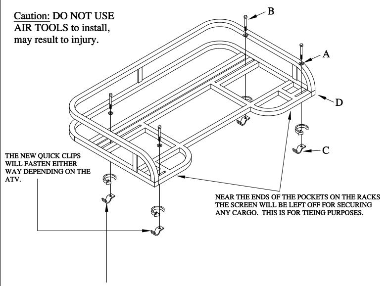
THIS CLIP WILL BOLT THROUGH THE FLAG POLE HOLE IN THE REAR OF THE RACK.
