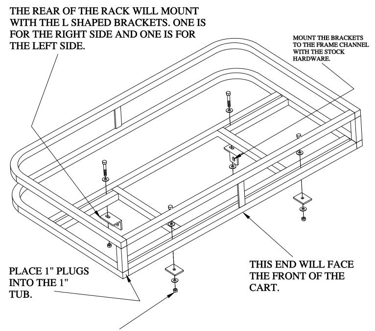
THE FRONT OF THE RACK WILL MOUNT IN THE 1" ROUND HOLES OF THE CHANNEL IRONS. PLACE THE SQUARE WASHERS UNDER THE CHANNEL IRONS.
