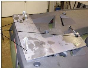
PLACE THE 569 BRACKETS ONTO THE REAR RACK. WILL HAVE TO REMOVE THE STOCK BOLTS ON THE REAR RACK WHERE THE HOLES FALL. CAUTION: THERE IS SPACERS UNDER THE RACK ON TOP OF THE FENDER MUST USE THESE TO MOUNT BRACKETS. REPLACE THE STOCK BOLTS WITH THE SUPPLIED COUNTERSINK BOLTS. REFER TO DRAWING FOR BOLT PLACEMENT.
