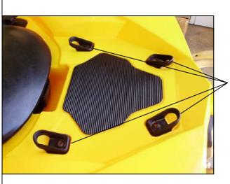
THEN REMOVE THE TIE BRACKETS ON THE REAR RACK. THESE CAN BE INSTALLED IN MANY PLACES ON THE NEW FLAT RACK....
