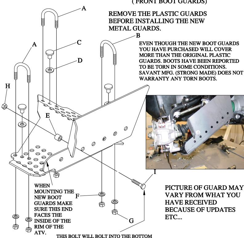
SHOCK EYE REMOVE STOCK BOLT AND REPLACE WITH THE 60MM BOLT AND NUT.
