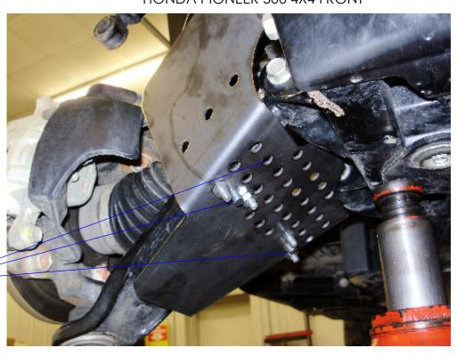
THIS IS THE PIC AFTER IT HAS BEEN MOUNTED THE BENT LIP WILL ALWAYS FACE THE FRONT DIFFERENTIAL.
