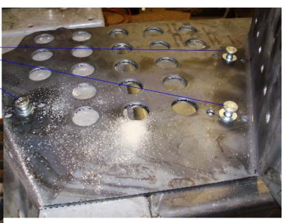
2ND STEP PLACE THE GUARD UNDER THE CONTROL ARM AND INSERT THE UBOLTS OVER TUB. INTO MOUNTING HOLES. THIS PROCESS IS MUCH EASIER IF THE WHEEL IS REMOVED.
