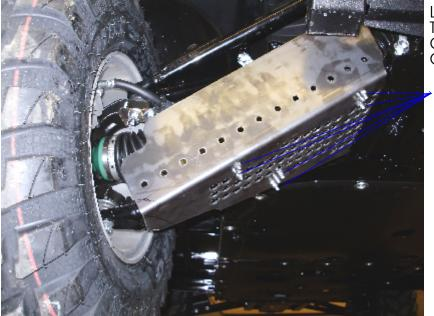
THE NEW GUARDS THAT YOU HAVE PURCHASED WILL COVER MORE THAN THE ORIGINAL PLASTIC GUARDS. BOOTS HAVE BEEN REPORTED TO BE TORN IN SOME CONDITIONS. DUE TO TIGHTER TURNING RADIUS ON SOME OF THE NEWER ATVS. THE GUARDS HAVE BEEN MANUFACTURED TO BE SMALLER. STRONG MADE **DOES NOT** WARRANTY ANY TORN BOOTS.
