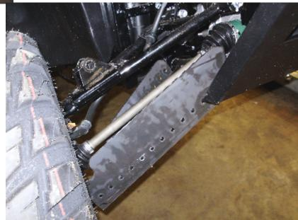
LAST STEP PLACE 1/4 LOCK NUTS ONTO EACH THREAD AND SECURE THE GUARD TO ARM. BE CAREFUL TO NOT OVER TIGHTEN GUARD AND CAUSE BENDING OF GUARD.
