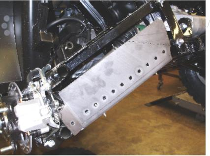
THIS IS A PIC OF THE REAR LEFT GUARD MOUNTED TO ARM. REPEAT SAME PROCEDURE FOR THE RIGHT SIDE.
