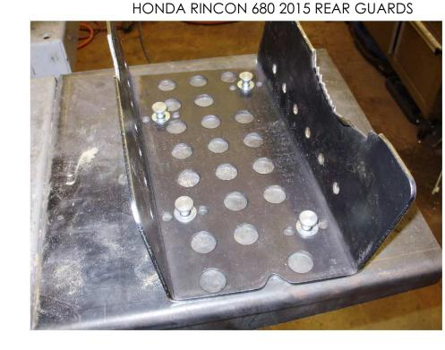
PLACE GUARD UNDER THE ARM WITH THE WASHERS AND RIVETS INTO POSITION. SLIDE IT DOWN TILL TOUCHES ROUND PIPE ON ARM. INSTALL THE UBOLTS AROUND THE TUBE OF ARM AND THREAD THE LOCK NUTS ONTO UBOLTS. TIGHTEN ALL HARDWARE.
