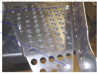
PLACE THE GUARD UNDER THE ARM LINE THE HOLES UP WITH THE THREADED TABS. THE ONE ON THE TOP LEFT IS NOT THREADED YOU WILL USE THE 1/4X11/4 BOLT 1/4 WASHERS AND LOCK NUT HERE.
