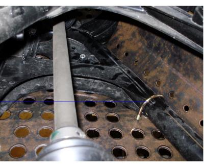
SECURE THE END OF THE GUARD WITH THE 1/4X1 1/2 BOLTS AND USE THE 3/8" SPACERS IN BETWEEN THE GUARD AND ARM ON THE INSIDE.
