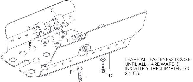
THIS IS A PIC OF THE REAR LEFT. THE REAR RIGHT WILL MOUNT THE SAME. BUT THE REAR BEND ON THE GUARD WILL BE SHORTER.
