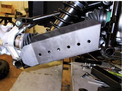
FINISHED PICTURE OF THE GUARD ONCE MOUNTED TO THE ATV. THIS IS THE LEFT REAR. ONCE MOUNTED MAKE A SHORT RIDE AND CHECK THE GUARD AND WHEELS TO MAKE SURE NOTHING IS TOUCHING OR RUBBING FROM THE TRAVEL OF THE SUSPENSION.
