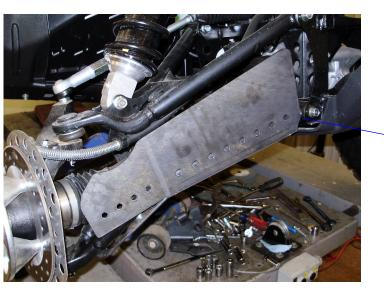
PLACE THE GUARD UNDER THE ARM LINE THE HOLES UP WITH THE THREADED TABS. USE THE 6MM BOLTS WITH 1/4 USS WASHERS TO THREAD INTO THE WELDED NUTS ON THE ARM.
