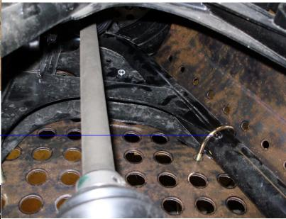
SECURE THE END OF THE GUARD WITH THE 1/4X1 1/2 BOLTS AND USE THE 3/8" SPACERS IN BETWEEN THE GUARD AND ARM ON THE INSIDE.
