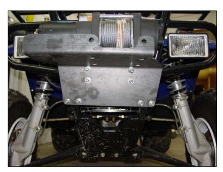
THE WINCH WILL HAVE THE HARDWARE TO MOUNT TO THE PLATE.
