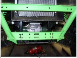
USE FOUR OF THE 5/16 X 1 1/4 BOLTS 5/16 WASHERS AND 5/16 LOCK NUTS TO MOUNT THE PLATE TO THE BUMPER. MOUNT THE LIP OF THE PLATE ON THE BACKSIDE OF THE BUMPER BRACE.
