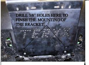
TO MOUNT THE SUPPORT BRACKET UNDER THE MAIN PLATE. USE THE TWO 6MM BOLTS, 1/4 USS WASHERS, TWO 5/16 BOLTS FOUR 5/16 WASHERS AND 5/16 LOCK NUTS. MUST DRILL TWO 3/8" HOLES FOR THE TOP HOLES IN THE SUPPORT BRACKET.
