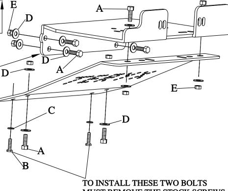
TO INSTALL THESE TWO BOLTS MUST REMOVE THE STOCK SCREWS THAT HOLE THE BOTTOM PART OF THE PLASTIC BUMPER GUARD.
